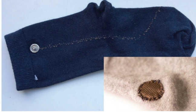
FIGURE 6.1. The smart sock and inlay of a fabric sensor.
