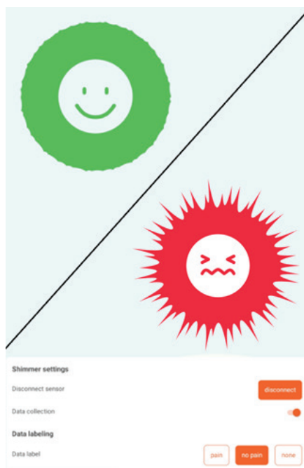
FIGURE 7.2. The user interface and visualization design of the SID Pain App when it is in use and gathering data. The green face is shown in case of no pain, the red face in case of pain.
