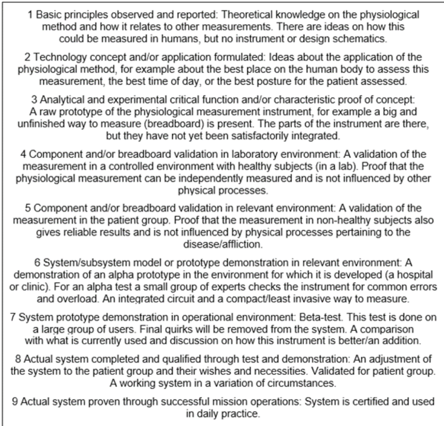
FIGURE S2.2. Technology Readiness Levels as described by the United States Department of Defense in accordance with instruments for physiological measurements of pain.
